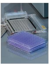
Automated vacuum filtration system for non-magnetic bead separation and DNA purification
