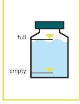
Liquid level detection (LLD) system to monitor bottle filling levels
