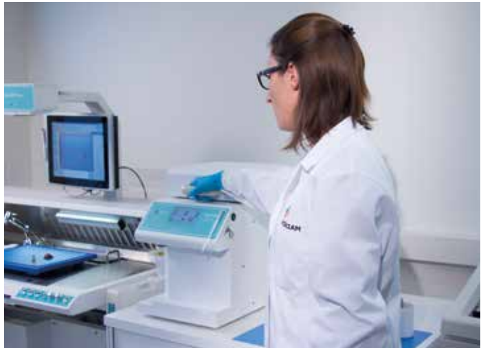
PrestoCHILL - Benchtop cryoembedding station
