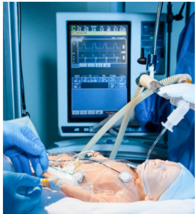
Premie HAL connected to a mechanical ventilator using a standard patient circuit.
