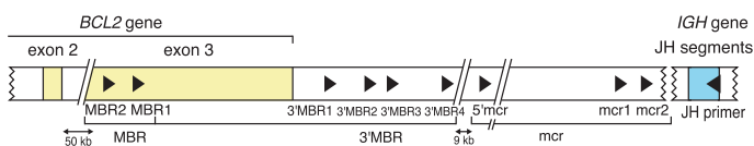
Figure Legend: Schematic diagram of the IGH-BCL2 t(14;18) translocation showing the BCL2 gene on the left and the Ig heavy chain ( IGH ) gene on the right. Shown are the relative positions and orientations for the major breakpoint region (MBR) primers, the minor cluster region (mcr) primers, and the J H primer, which are included in the 3 BCL2 / J H master mix tubes.
