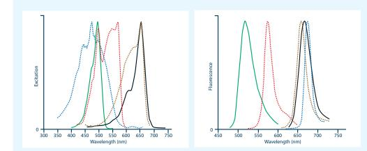
**Figure 1.** Excitation (left) and emission (right) spectra of Alexa Fluor® 488/FITC (green), R-PE (red), PerCP (blue), Alexa Fluor® 647 (black), and APC (brown). Peak heights were normalized after the spectra were obtained with an M-series spectrofluorometer system from Photon Technology International, Inc.
