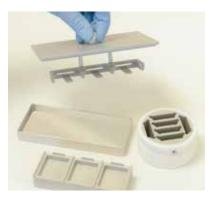
1 The cryomold kit (optional) allows to carry out standardized flash freezing.
