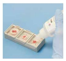
**3** Fill the cryomold with the Milestone MCC compound.
