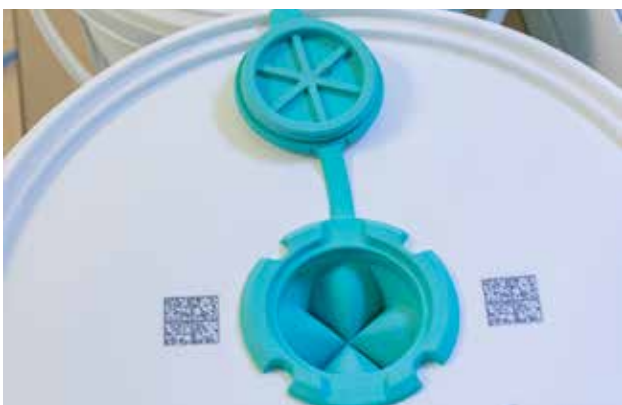
Quadricuspid valve during operation
