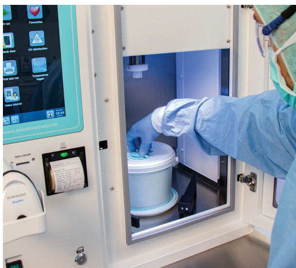
Figure 2. Example of an automatic formalin dispensing system inside a protected area.
