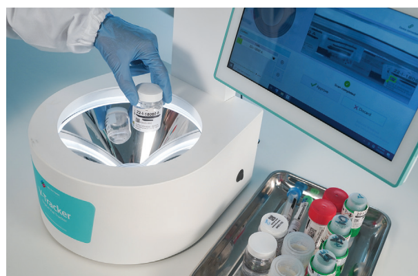
Figure 7. Example of automatic accessioning tracking system.
