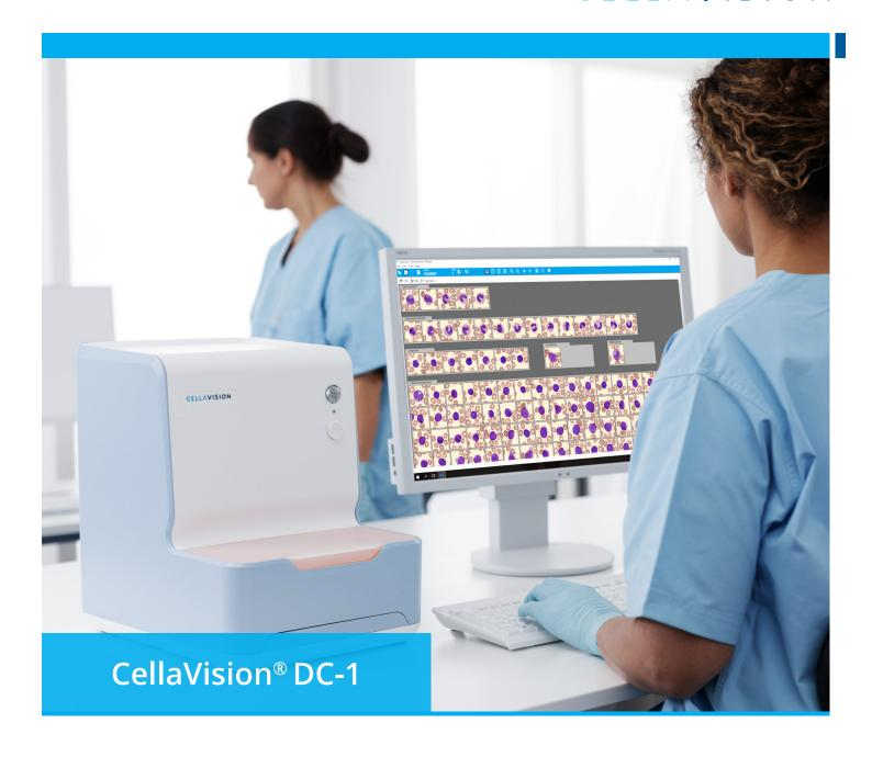
The CellaVision DC-1 is designed to automate and simplify the process of performing blood cell differentials in low-volume laboratories. The system leverages high-speed robotics and digital imaging to automatically locate and capture high quality images of cells. It allows both **stand-alone** and **networked installation**.
