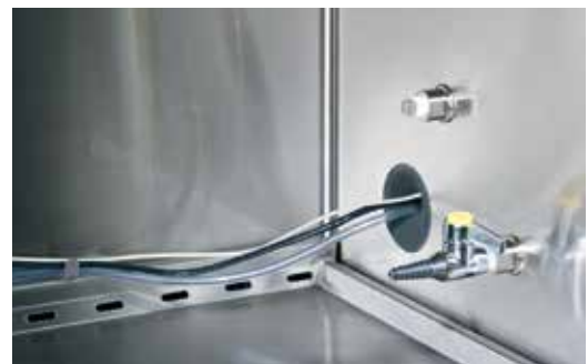
Patent-pending, NSF-approved cable port on right allows cables and/or tubing to exit cabinet side walls rather than front work area, eliminating obstructions, hazards, and interference with proper viewscreen closure.
