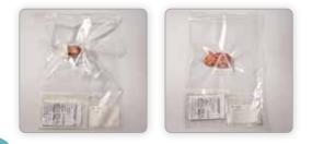
Specimens are placed in single use special vacuum bags and sealed by closing the
