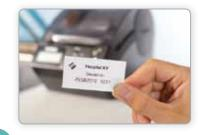
**Documenting time of sealing** At the push of the button a label is printed with name of hospital, date and time. The label is affixed through the sealed bag.
