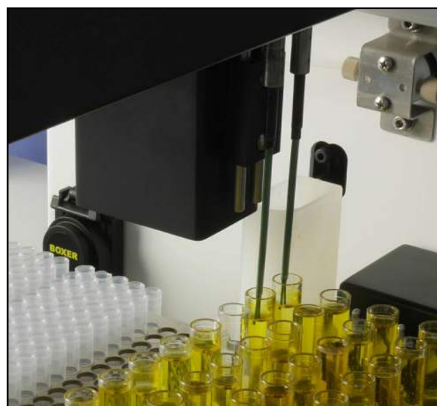
Dual nozzle probe aspirating sample
