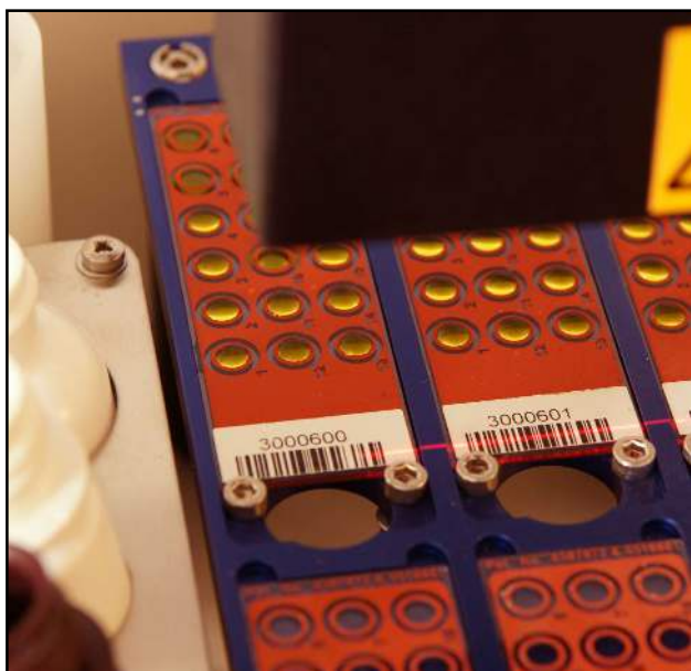
Linear barcode reader acquiring barcodes from slides
