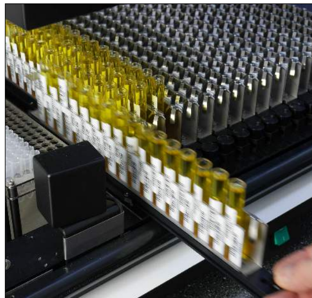
Barcode reader acquiring 1D barcodes from sample tubes minimum.
