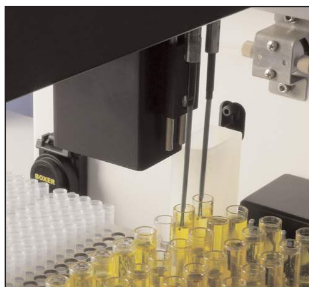
Dual nozzle probe aspirating sample
