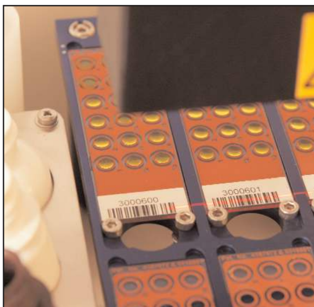
Linear barcode reader acquiring barcodes from slides
