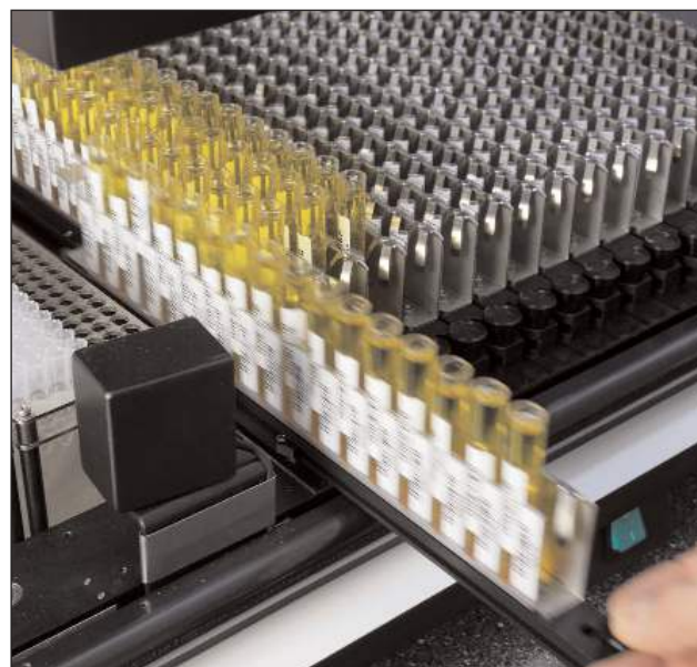
Barcode reader acquiring 1D barcodes from sample tubes
